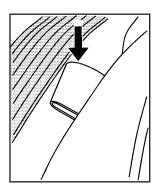
Pull forward on the tab, located on the outboard side of the seatback, to unlock the seatback.
